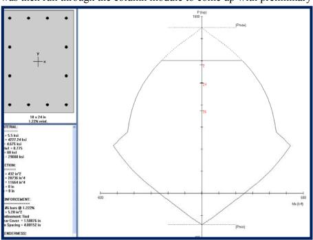
The rebar layout for all columns are (12) #6's arranged with 4 on the 18" faces and 2 in between on each side. Column designs were also spot checked with PCA Column.
