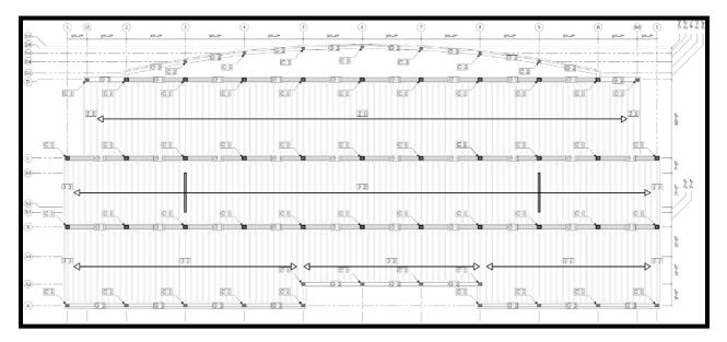
The CRSI Design Handbook was used to do the preliminary design. The design was picked based on the length of the span, superimposed load, and moment. This resulted in the selection of 30" wide forms with 6" ribs and a total slab depth of 24.5", 20" ribs with a 4.5" slab depth. This 4.5" slab gave the system its desired two hour fire rating. Rebar was then sized based
